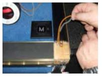
Connect the IAV led wires into the supply, red joined into the red and black into the black cables
